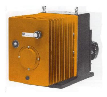
Make: Alcatel Model: 2100A Displacement: 120 CMH Stages: 2 *Type of oil: H/C* Inlet connection: KF50 Outlet connection: Motor power: 3 kW 415 V 3 Phase Gas ballast: Yes Cooling: Air Weight: 235 Kg Length: 958 mm Width: 344 mm Height: 588 mm Accessories available: **Oil Mist Filter Oil Filtration Unit**
