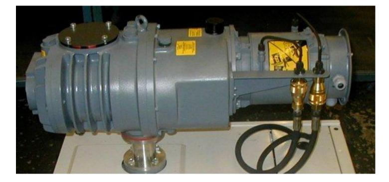
Make: Edwards Model: QMB250 50 Hz Part No. A301-85-905 60 Hz Part No. A301-86-905 Displacement: 250CMH Inlet connection: ISO63 bolted Outlet connection: ISO40 bolted Type of oil: PFPE Minimum size backing pump: 40 CMH Motor power: 1.5kW, 415 V, Three Phase Cooling: water Weight: 65 Kg Length: 700 mm Width: 270 mm Height: 292 mm
