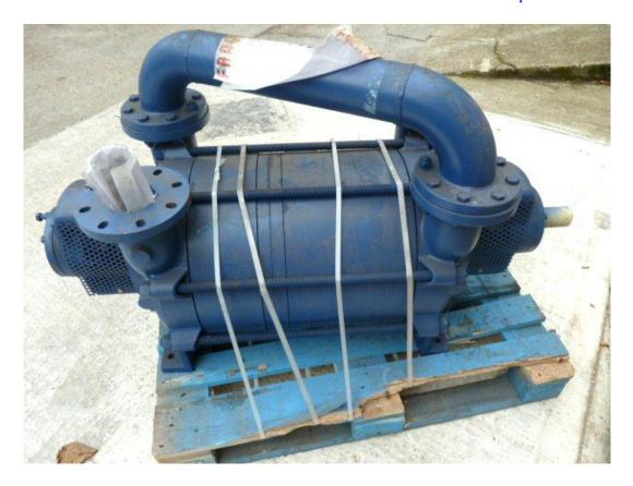
Make: Edwards Model: LR2S1250 – Bareshaft Part No. A75154986 Displacement: 1250 CMH Vacuum: 33 m/bar Pressure: N/A Inlet connection: ANSI **Outlet** connection: ANSI Motor power: 37kw Type of oil: N/A Weight: Length: mт Width: mm Height: mm
